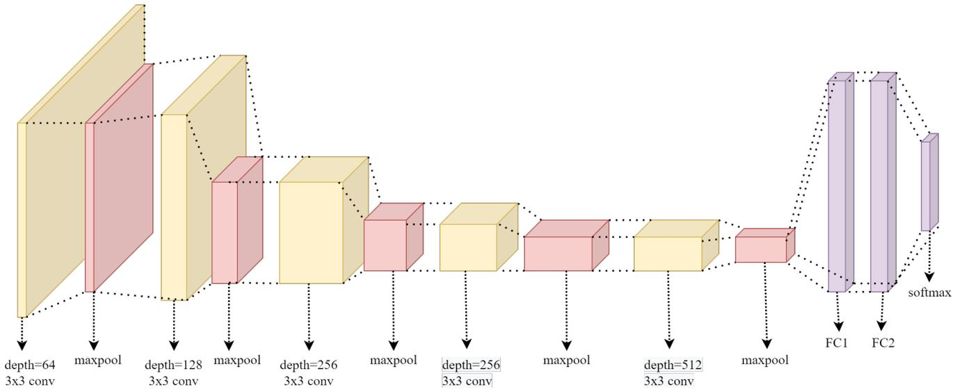
Fig. 1. The 19 layers of VGG19 network used for feature extraction. This architecture was initially proposed by Simonyan *et al.* in [7]
