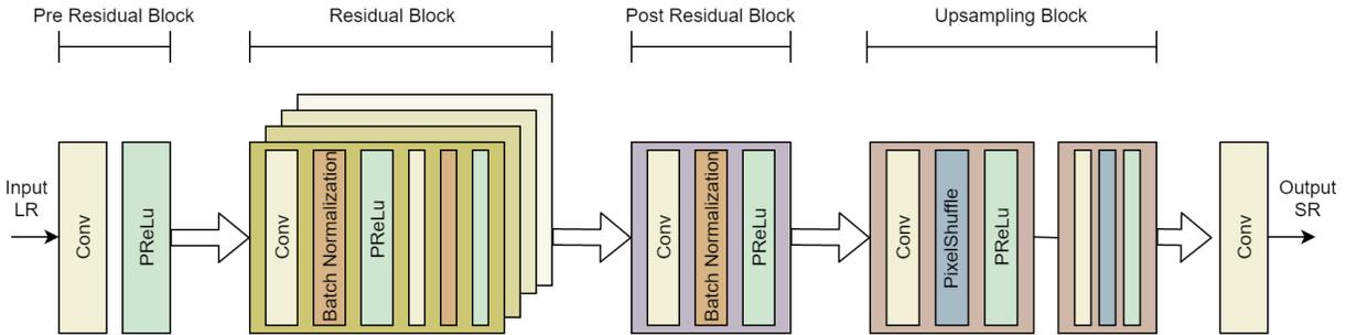
Fig. 2. Architecture for Generator network.
