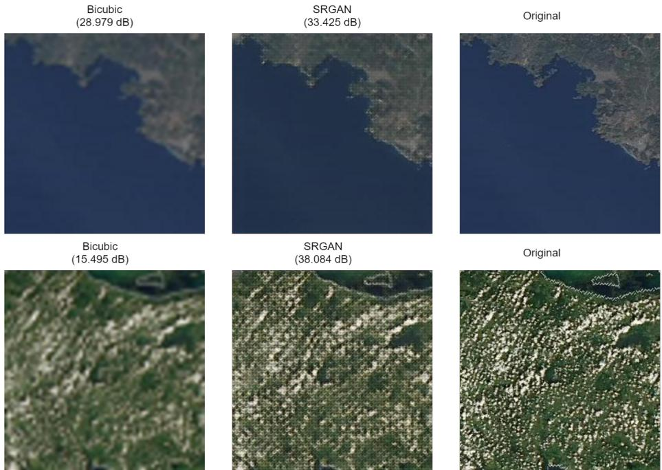
Fig. 6. PSNR evaluation of SRGAN for MODIS dataset with 250m spatial resolution. Right: original images that are down-scaled by a factor of four. Middle: SRGAN reconstruction form down-scaled image. Left: Bicubic interpolation reconstruction from down-scaled image. Top and Bottom are different satellite readings.
