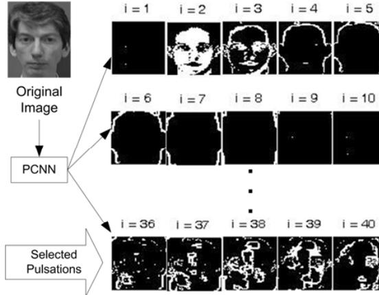
Fig. 2. Images pulsed by a PCNN when a face image is the input. Pulsations 36 to 40 are selected as features.
