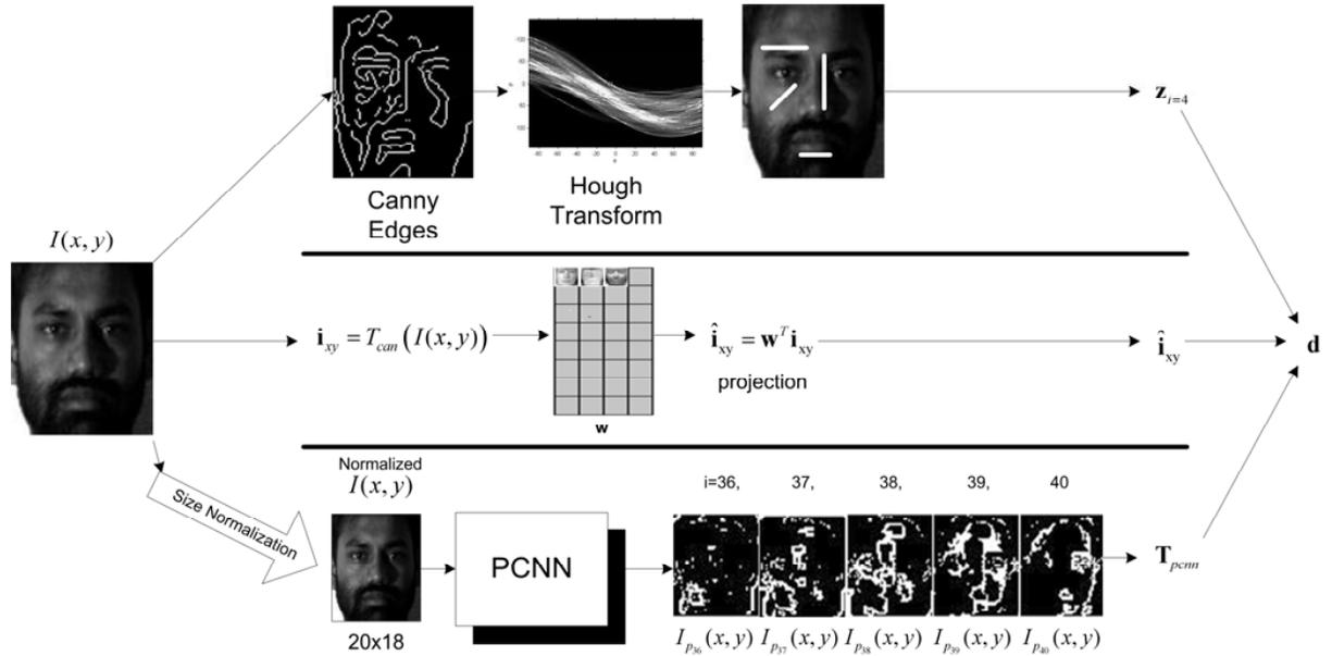
Fig. 4. Feature extraction method. First the Face Feature Lines, FFL, are calculated and placed in  $\mathbf{Z}_{i=4}$ ; second, uncorrelated features are extracted with KLT method and placed in  $\hat{\mathbf{i}}_{xy}$ ; third, the PCNN approach is computed and the pulsed images are stored in  $\mathbf{T}_{pcnn}$ . All the features are concatenated into the vector  $\mathbf{d}$ .
