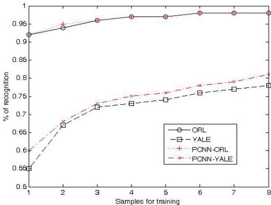
Fig. 11. Comparison of the experiments realized on ORL and YALE face databases with/without PCNN.
