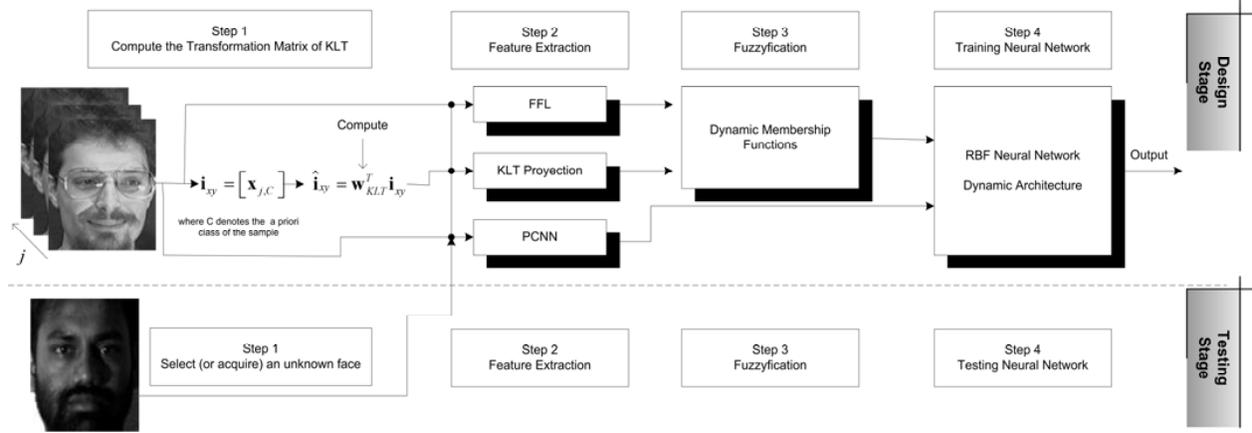
Fig. 8. Stages of the proposed system. This figure shows the similarity of the Design and Testing stages, and illustrates the overall process.
