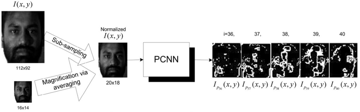
Fig. 3. Reduction via sub-sampling, and magnification via averaging, from two different image sizes.
