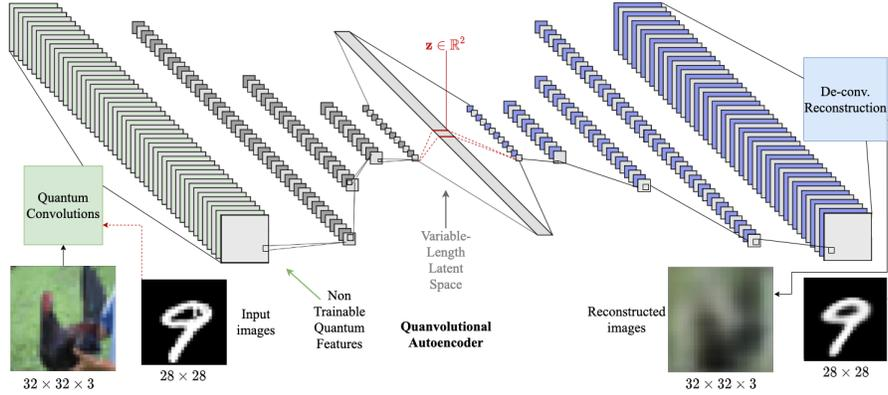
**Fig. 2.** *Top:* Quanvolutional autoencoder architecture, where the quantum filtering (quantum convolutions) are described as quantum circuits, as shown in Fig. 3. The quantum layer is non-trainable by the network. *Bottom:* Classic convolutional autoencoder with all its layers trainable. Note that the dense layer in the center of the AEs can also vary, producing a two-dimensional latent space or a larger space.
